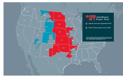
SPP has a footprint that spans nearly 575,000 square miles in the central United States and includes more than 800 generating plants, nearly 5,000 substations and about 56,000 miles of high-voltage transmission lines.
