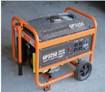
Backup generators can turn into lethal hazards for lineworkers if they are not connected properly.
